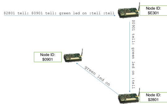
Fig. 3: Recursive employment of the tell: primitive. Once the node with ID E301 encounters the first tell: it parses all the following symbols until the last :tell and a frame containing 0901 tell: green led on :tell is sent to node with ID 2801. The payload interpretation of the payload on the receiving side leads to the sending of a new frame destined to node 0901 with green led on as payload. Once received, node 0901 turn its green LED on.
